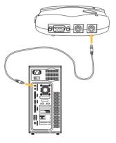
Repeat Steps 1 through 3 for each additional computer to be connected to the Switch, connecting them to the corresponding CPU ports on the side.
